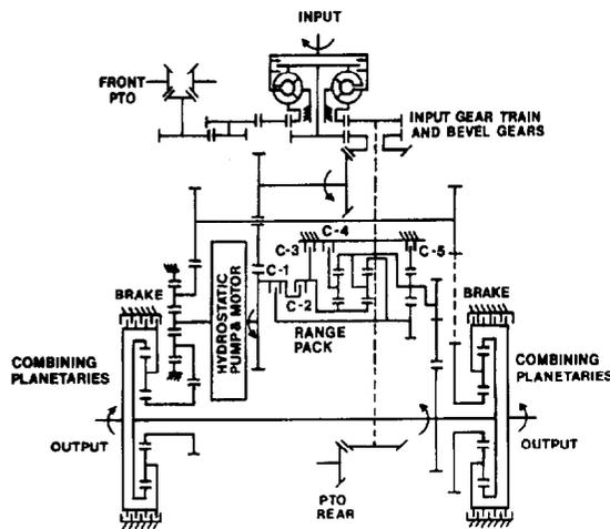
Fig.3 Hydrokinetic Transmission
