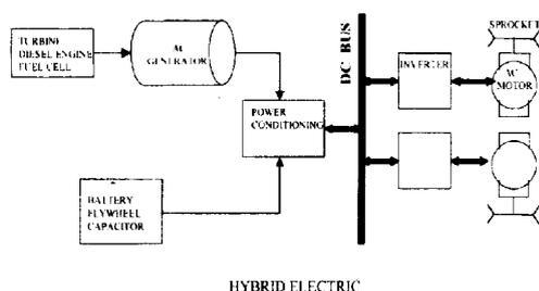
Fig.6 Electric drive schematic
