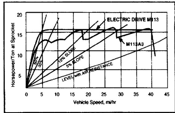
Comparison of available horsepower for the M113A3 and the Electric Drive M113 at same engine rating
